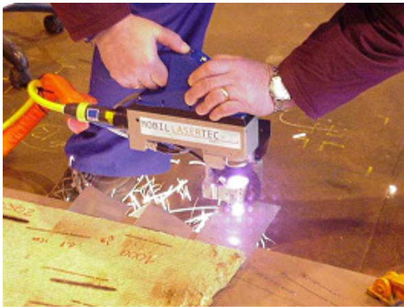
hand guided device for cutting and welding – here: cutting
